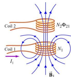
**Figure:** Changing current in coil 1 produces changing magnetic flux in coil 2.
