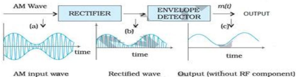
Block diagram of a detector for AM signal.
