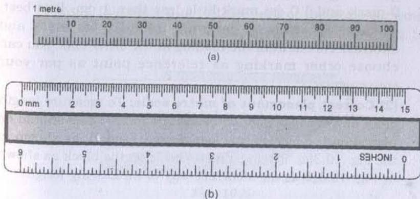
**Fig. 10.1** Correct metre scale (a) A metre scale and (b) A 15 cm scale
