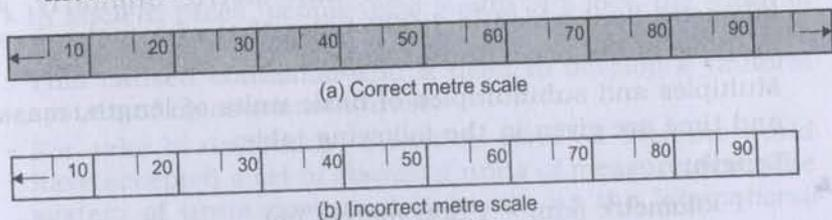
Fig. 10.2 Correct use of metre scale
