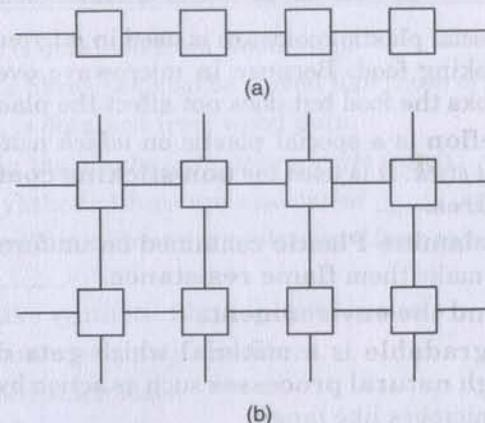
Fig. 3.1 (a) Linear (b) Cross-linked arrangement.
