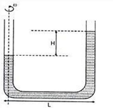
3. A U-shaped tube contains a liquid of density  $\rho$  and it is rotated about the line as shown in the figure. Find the difference in the levels of liquid column.
