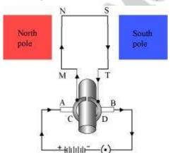
When a current is allowed to flow through the coil MNST by closing the switch, the coil Contact us: info@emedicalprep.com | +91-120-4616500 starts rotating anti-clockwise. This happens because a downward force acts on length MN
