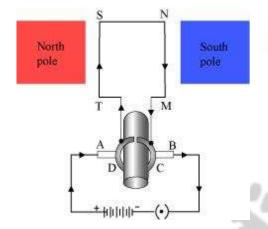
The current flows through the coil in the direction TSNM. The reversal of current through the coil MNST repeats after each half rotation. As a result, the coil rotates unidirectional. The split rings help to reverse the direction of current in the circuit. These are called the commutator.
