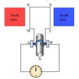
In this arrangement, brush **A** always remains in contact with the length of the coil that is moving up whereas brush **B** always remains in contact with the length that is moving down. The split rings **C** and **D** act as a commutator.
