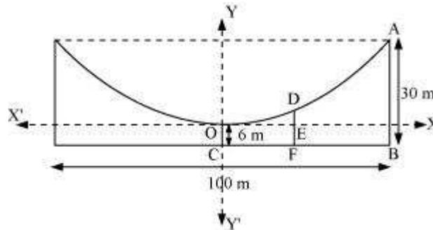
Here, AB and OC are the longest and the shortest wires, respectively, attached to the cable.
